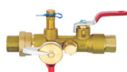
UB VALVE Size 1/2" - 2", Max. 600 psi, @ 250°F Shut-off, optional unions and multiple accessory ports (Shown with optional accessories)
