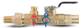
UA VALVE Size 1/2" - 2", Max. 600 psi, @ 250°F Balancing, union, shut-off and optional port
