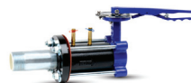
WT VALVE Size 2-1/2" - 3", Max. 200 psi, @ 250°F Flow regulator, shut-off and dielectric nipple (Designed to attach directly to brass-body threaded ATC)
