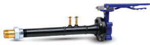
ET VALVE Size 2-1/2" - 4", Max. 240 psi, @ 250°F Steel venturi, flow measurement, shut-off, dielectric nipple and extended inlet (five pipe diameter)
