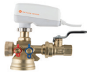
HARMONY VALVE Size 1/2" - 6", Max. 240 psi, @ 250°F Steel venturi, flow measurement, shut-off and reducing inlet flange
