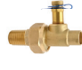
UP VALVE Size 1/2" - 2-1/2", Max. 400 psi, @ 250°F Union and port sections (Shown with optional pressure/ temperature port)
