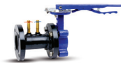
AF VALVE Size 4" - 16", Max. 340 psi, @ 250°F Flanged steel venturi, flow measurement and shut-off
