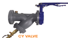
CY VALVE Size 2-1/2" - 8", Strainer, drain valve and shut-off CW - Max. 125 psi, @ 250°F BF - Max. 240 psi, @ 250°F
