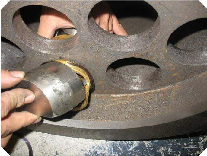
Remove the spring insert adapter out of the body.
