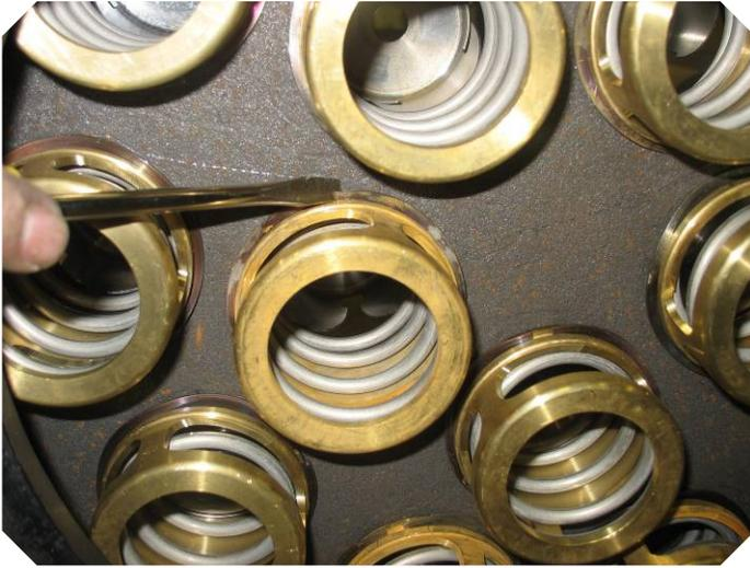
Place screwdriver on the gap and lift the spring out.
