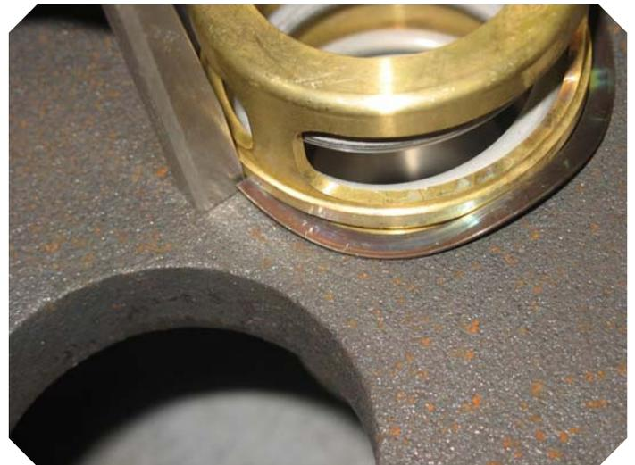
Recheck if the gauge goes into the gap as shown in the picture above.
