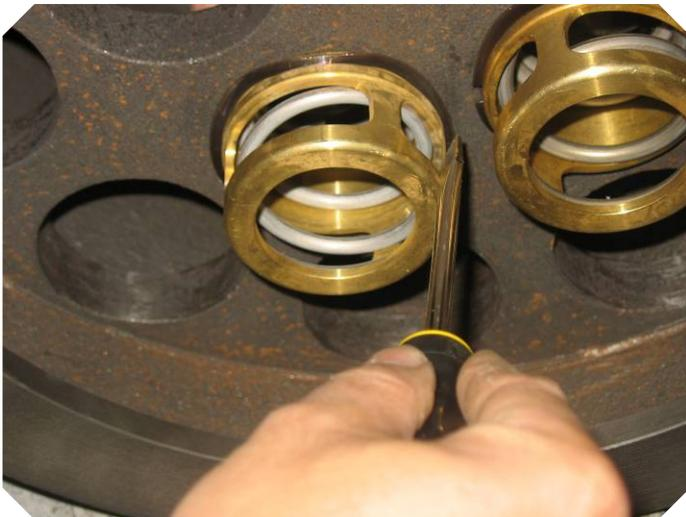
Make sure the spring is inside of groove.
