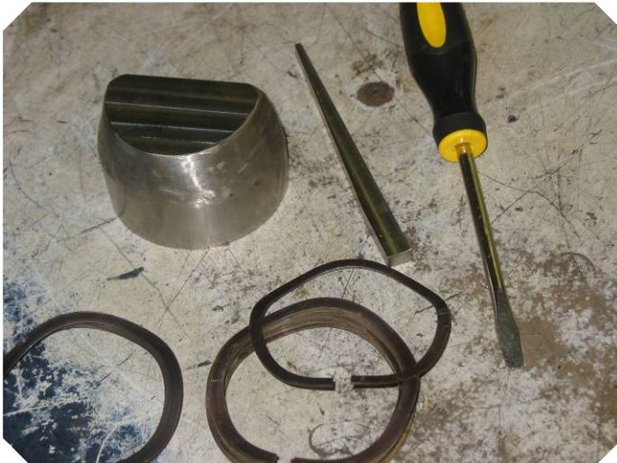
Flat screwdriver, spring insert adapter, no-go gauge.
