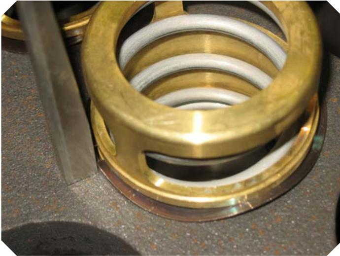
Wave spring is fitting correctly if the gauge doesn't go into the gap as shown in the picture above.
