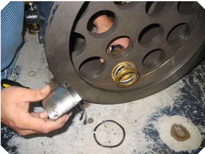
Insert canister assembly into WS body starting with the outer circle.
