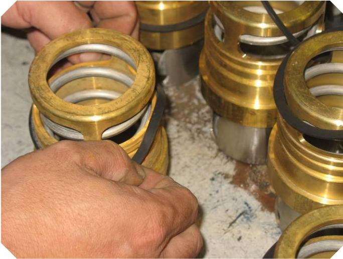
Insert gasket onto canister bottom.
