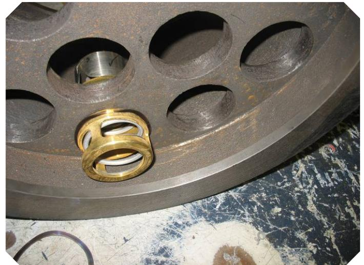
Wave spring is inserted within groove.
