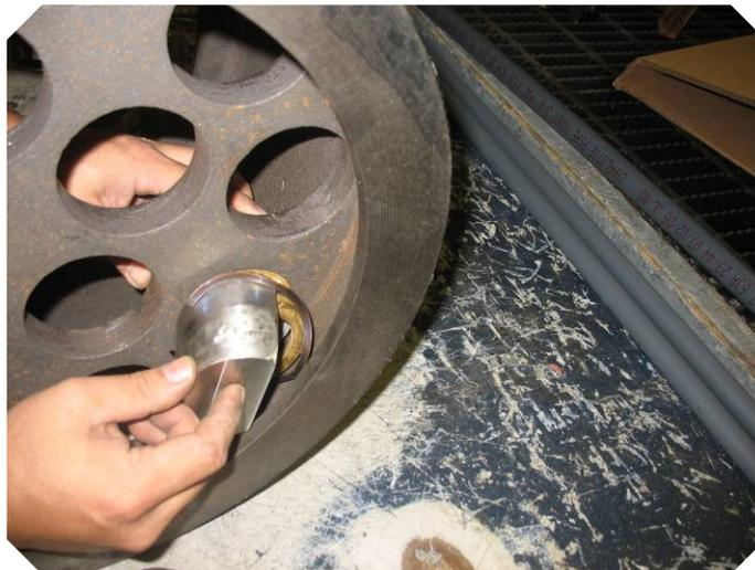
Use screwdriver to insert spring clip into groove.
