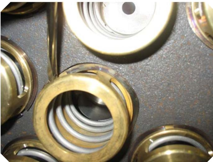
Take the spring out using a screwdriver as shown in the picture above.
