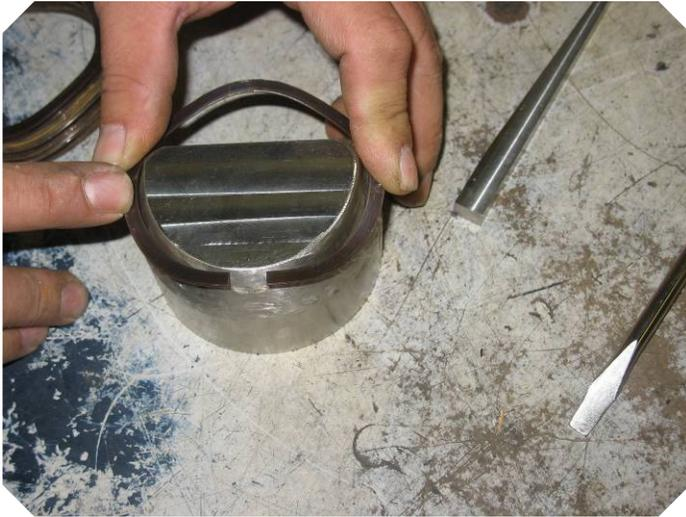
Place wave ring on tool with high side. The high side is shown in the picture when ends of spring are pointing up.
