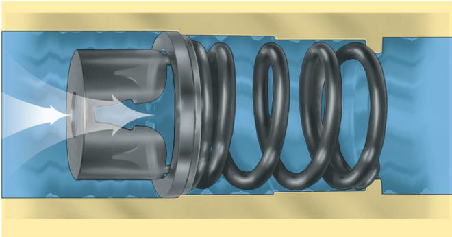
The differential pressure is below the minimum needed to activate the AutoFlow piston. It is fully extended and acts as a fixed orifice with a Cv of .71 times design flow (2-32 range) or .45 times design flow (5-60 range). The ATC is controlling the GPM in this zone.
