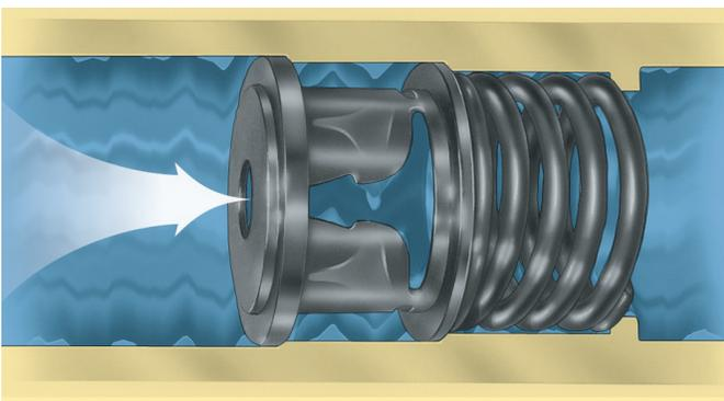
Now fully retracted, only the AutoFlow piston's end port is exposed. The regulator functions as a fixed orifice and will react to increased pressure differential with increased flow in accordance with the formula:  $GPM = C_v \sqrt{\Delta P}$ . Fixed Cv of the valve is now .18 times design flow (2-32 range) and .13 times design flow (5-60 range). A 25 percent "over range" (32 psi to 40 psi) increases the flow by only 12 percent!
