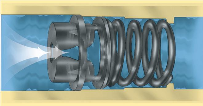
AutoFlow piston now responds to changes in differential pressure by repositioning the variable side orifices to maintain design flow  $\pm$  five percent. At approximately 50 percent of control range, the consolidated side port now handles all flow through the variable orifice. The Cv is variable in this range and is a function of piston position.
