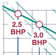
AutoFlow units save additional pump energy by preventing overflow compared to manually balanced two or three-way controlled coils. Modulating three-way valves can overflow by 40 percent and manually balanced two-way valves can overflow 20 percent to 30 percent when some of the valves are closed or at part load. As a rule of thumb, automatic balancing can save ten percent of the installed BHP when compared to a manually balanced system.
