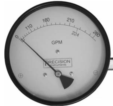
Example GPM meter for VFL400 0-260 GPM based on 75" WC with the 224.0 click marked.
